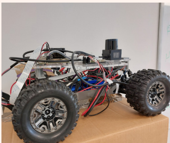
➤ MODEL OF AN F1/TENTH AUTONOMOUS CAR, OPERATING WITH A REAL-TIME SOFTWARE ARCHITECTURE, DEVELOPED BY THE SYCOMORES TEAM
